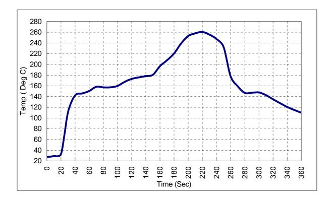
The components shall remain within the electrical specifications after it soldered on the 1mm thickness PCB board and dipped in the solder at  $260 \pm 5 \text{ degC}$  during  $10 \pm 1 \text{ seconds}$ .
