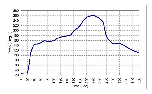
The components shall remain within the electrical specifications after it soldered on the 1mm thickness PCB board and dipped in the solder at  $260 \pm 5 \text{ degC}$  during  $10 \pm 1$  seconds.
